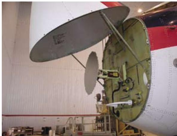
Installation of the E-Turb radar, a modified radar unit that can detect turbulence associated with thunderstorms by measuring the motions of the moisture in the air.
